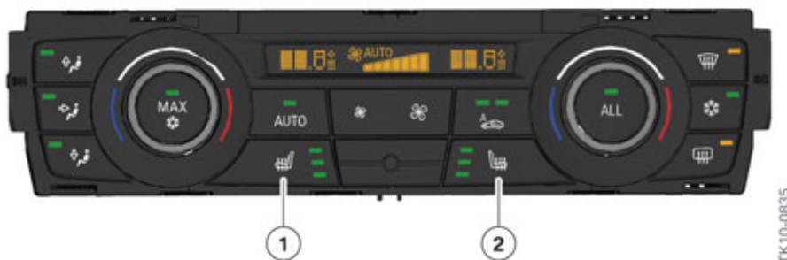
F25 IHKA control box
