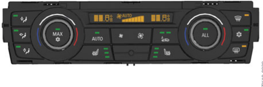
F25 Control panel of 2/1-zone IHKA
