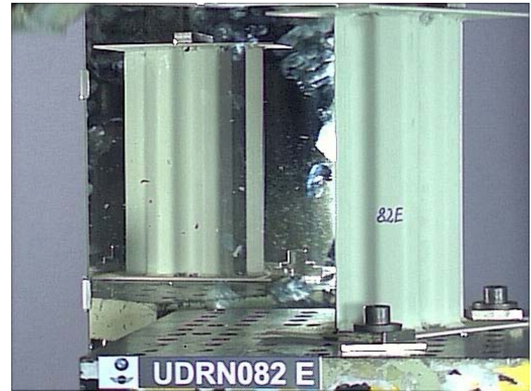
Specimen after Drop Test
