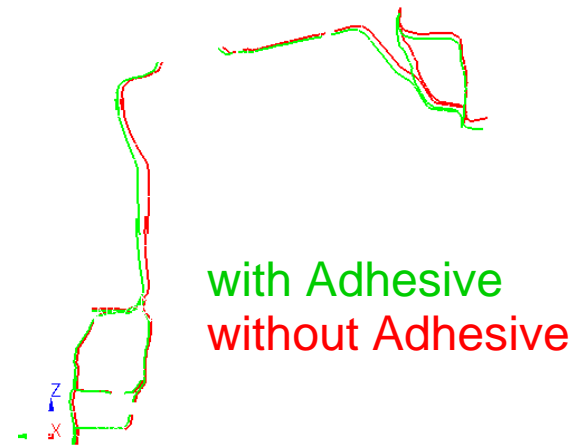
Difference of Displacements of the Spring Support with and without Adhesive Application
