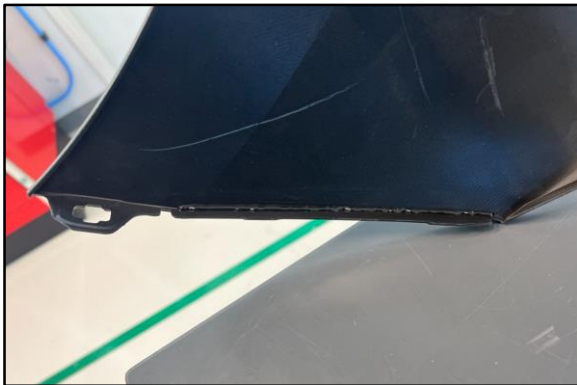
Figure 10. Left-hand Side Bead Applied
