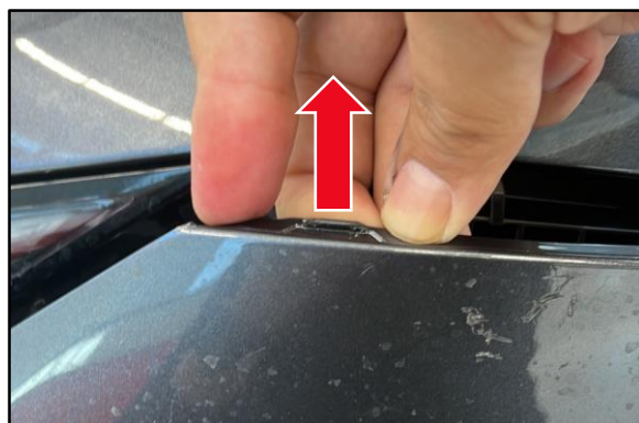
Figure 4. Tab During Adjustment
