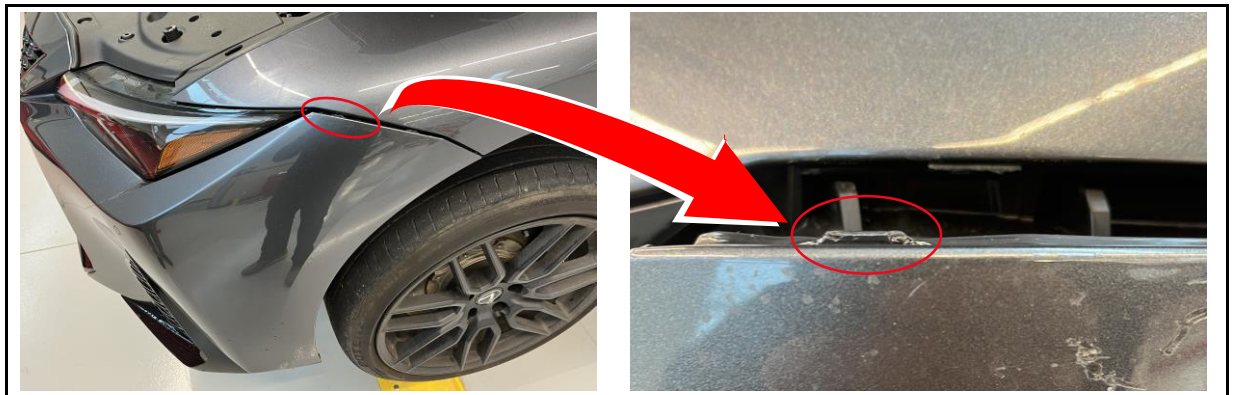
Figure 3. Tab Before Adjustment
